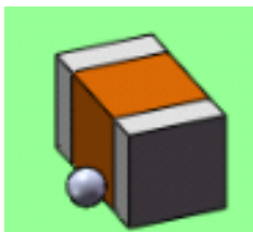
Figure 26 - Solder Ball on a Passive Package
