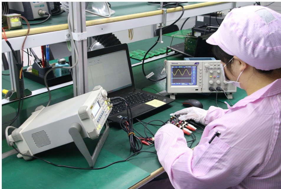
Figure 29 - GWT Test Engineer Performing FCT on an Assembled Board
