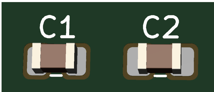
Figure 14 - Minimum Ratio (C1 - Left) & Larger Ratio (C2 - Right) – Both Acceptable
